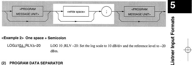
LOGA10A;RLVA-20 LOG 10 ;RLV -20: Set the log scale to 10 dB/div and the reference level to -20 dBm.
