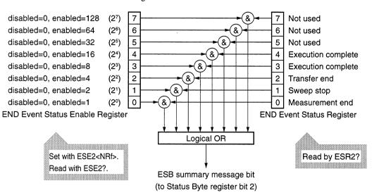
This section explains END event status register model operation and names and meanings of events.
