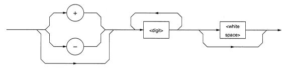
• 0 (s) may be added at the beginning. 005, + 000045  $\rightarrow$ • A space (+ or –) must not be inserted between a sign and a numeric.  $\rightarrow$  $+5, +\Delta 5 (\times)$ Spaces may be added after a numeric.  $+ 5\Delta\Delta\Delta$ •  $\rightarrow$ The + sign may be omitted. +5,5  $\rightarrow$ Commas must not be used to indicate decimal places. 1,234,567 (×) ۲  $\rightarrow$
