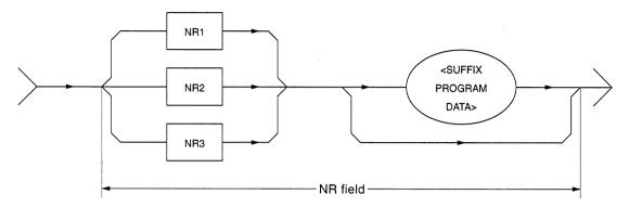
A suffix is added at the end of decimal numeric program data only when the data requires a unit of measure. It is a combination of a suffix unit and a suffix multiplier. The syntactical chart is shown below. Bold-line routes are used frequently.
